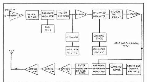
fig. 4. A look at single sideband in 1930, when it was hardly a household word! Because of the problem of building a high-Q sideband filter, the early transmitters started out with a balanced modulator in the 20 kHz to 50 kHz range. This circuit shows sideband generation in the 16-19 kHz range, with additional mixing to 265 kHz.
